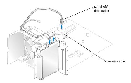
**3** Press in on the blue tabs on each side of the drive and slide the drive up and out of the computer.
