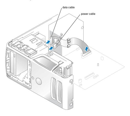
**5** Remove the CD/DVD drive by sliding and holding the drive release latch downward. Then, slide the drive out of the computer.
